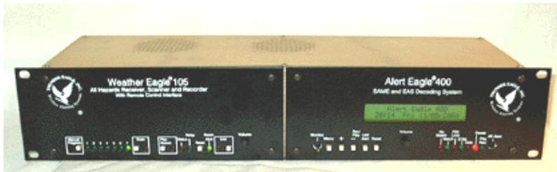
The AlertEagle®400 (AE400) is a high performance, patented, diagnostic EAS/SAME decoder. The AE400 system includes the Weather Eagle 105 radio receiver and the AE400 decoder. This system translates EAS/SAME encoded messages from NOAA's National Weather Service into readable text and relays that text by LAN/WAN and Internet to printers, email and pagers. The system is designed in a modular fashion so that parts of the system can be added as your budget permits.
